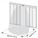
Mounting height 2200 mm / tilt angle  $30^\circ$  Antenna position:
